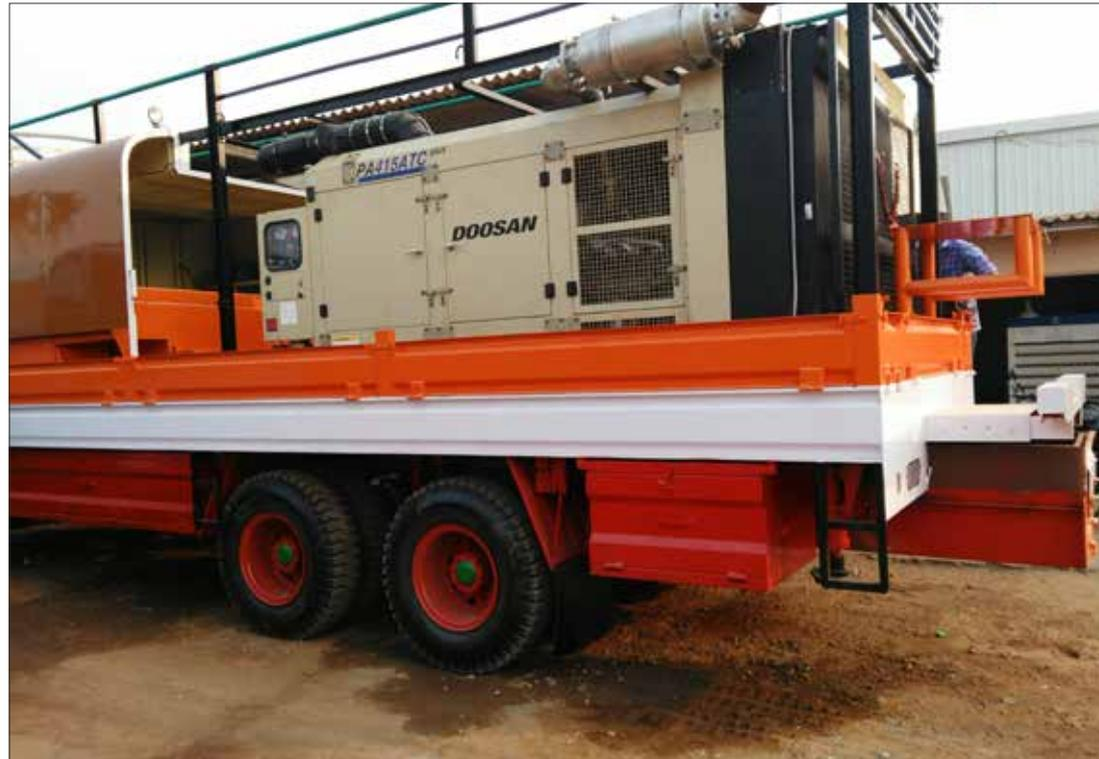
Pictured here is a truck mounted companion pneumatic air compressor with a 2,800-liter on-board fuel tank. Once these machines drop anchor at a drilling site, they often drill continuously for 48-72 hours. Each drilling operation may consume up to 2,000 liters of diesel fuel. The Nearest gas station may be 100 km away. Manual refueling is done onsite using portable barrels & jerry cans.
